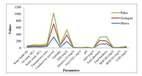
Figure 1. Average variation in the physicochemical parameters of water.
