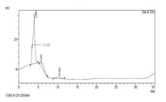
Figure 1. HPLC chromatograph of methanolic extract of Azadirachta indica.
