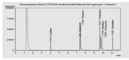
Figure 1. Typical chromatograms of seven organophosphorus insecticide standards run by GC-FTD.
