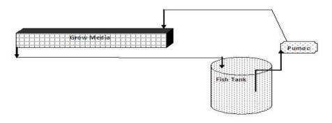
Figure 3. Small scale and media based aquaponics system used in our present study.
