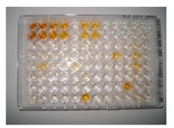
Figure 5. Enzyme Linked Immuno-sorbent Assay; Positive test showing reddish color no. F10 and G6.
