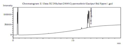
Figure 5. Chromatogram of cypermethrin standard solution.
