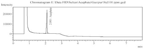
Figure 3. Chromatogram of acephate standard solution.
