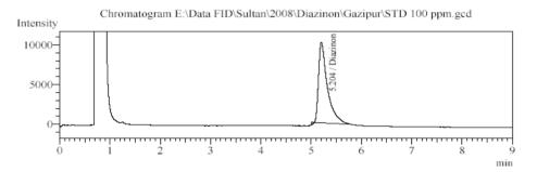
Figure 1. Chromatogram of diazinon standard solution.
