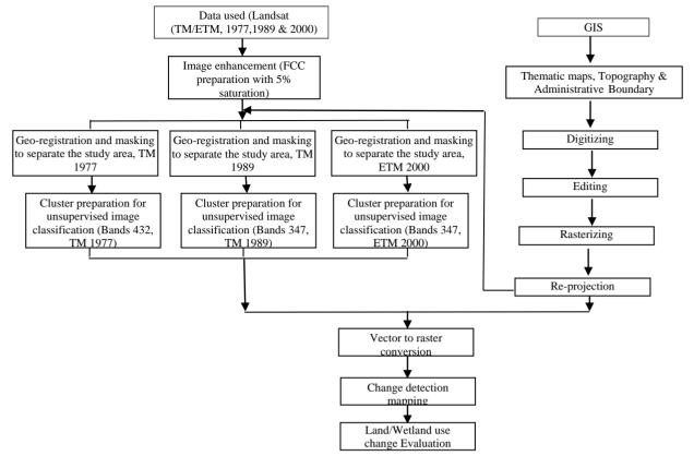
Figure 2. Schematic diagram of the major steps of image processing techniques adopted in the study.
